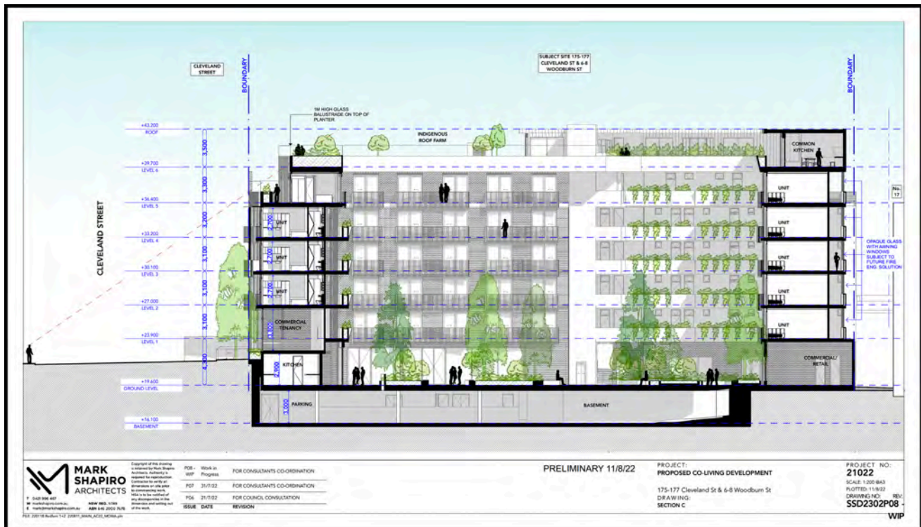
Figure 2 – Generic north-south section through proposed design – from MSD Architects
