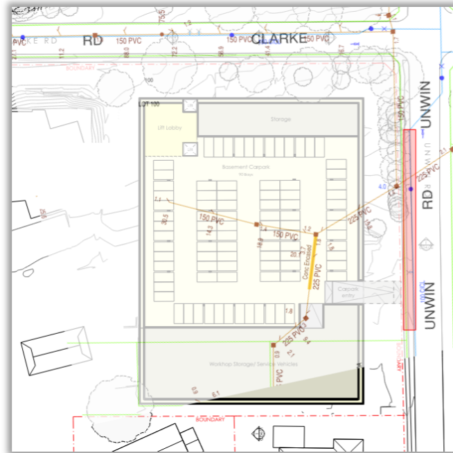
Figure 6.6.2 – Recital Hall – water main adjacent to building Unwin Road
