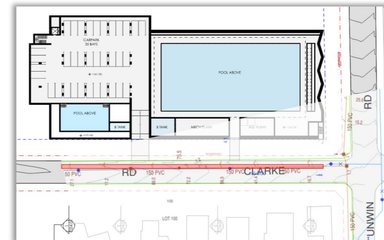
Figure 6.6.1 – Aquatic centre - water main adjacent to building Clarke Road
