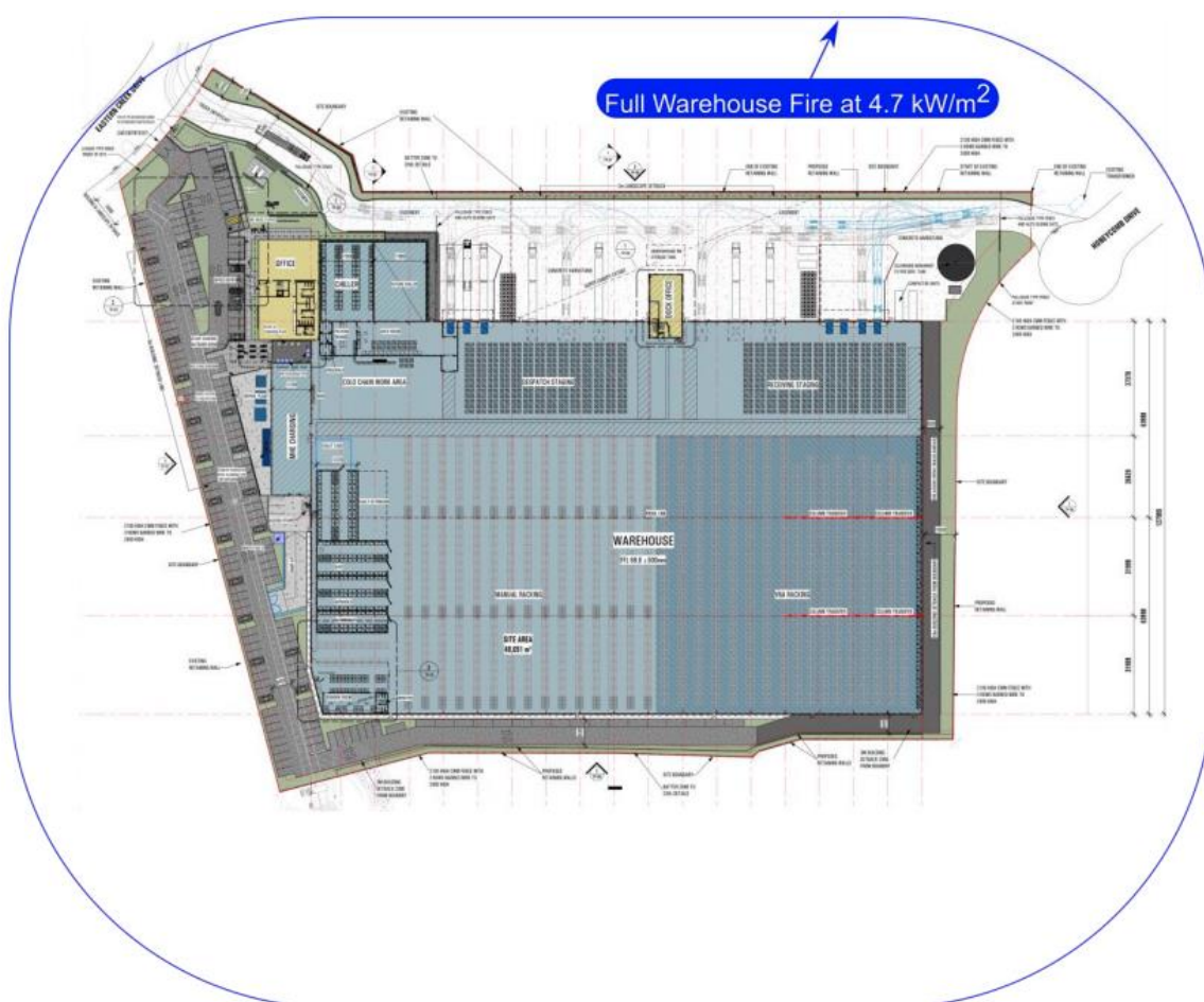
Figure 50 Full Warehouse Fire Radiant Heat Contours (Source: Riskcon, 2022)
