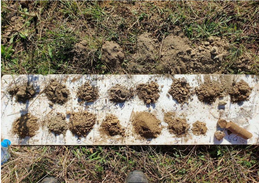
Photo 5 - Typical Soil Profile at BH01 (25/5/2022)
