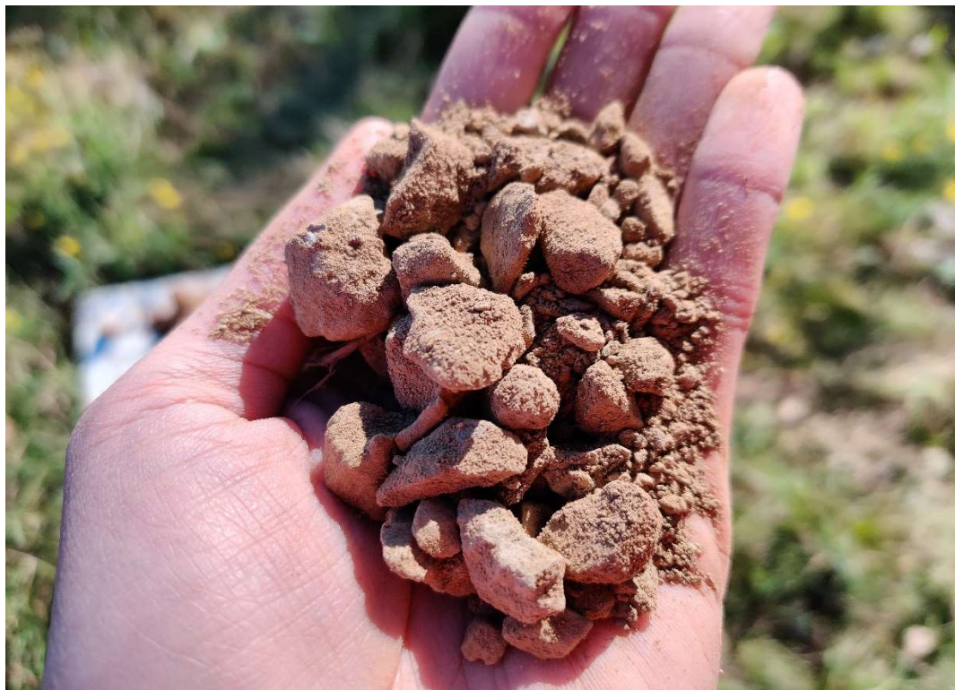
Photo 6 - Typical Bedrock (SHALE) Material at BH03 (08/6/2022)
