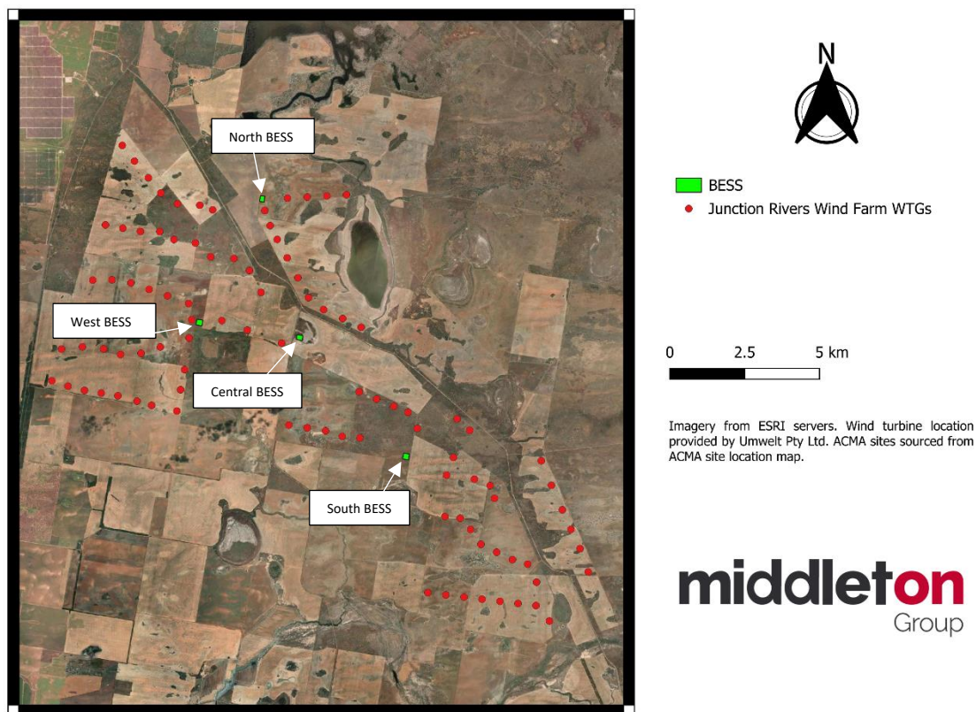
Figure 11: The Project BESS Layout
