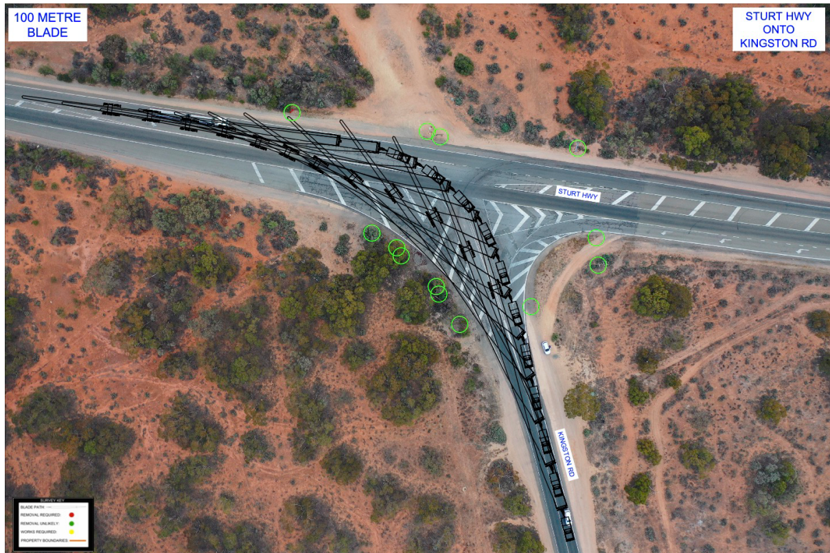
Figure 19 - Sturt Highway onto Kingston Road at Kingston, SA.
