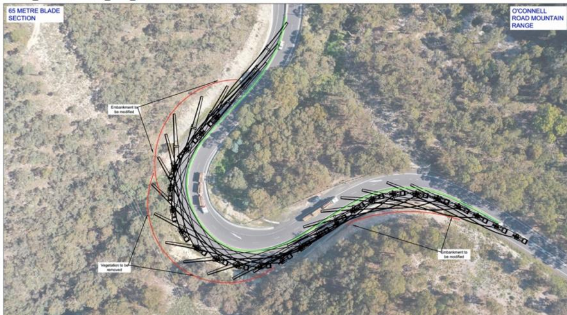
Figure 2 – An example of one road modification that will be required on O’Connell Rd for the Paling Yards Wind farm - taken from the EIS Route Study – Newcastle to Paling Yards.
