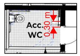
Additionally, it is noted that only a single ambulant sanitary compartment is proposed for the staff facilities. As part of the BCA Report, it is required that two of these WCS are allocated to Female and one WCs is allocated to male. Therefore, it would be required that there are two ambulant facilities provided in accordance with AS1428.1-2009.
