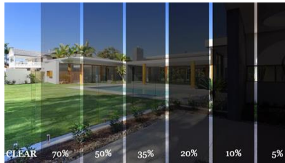
Figure 3 Indication of VLT glazing tints
