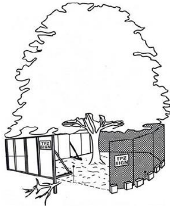
Tree protection fencing
