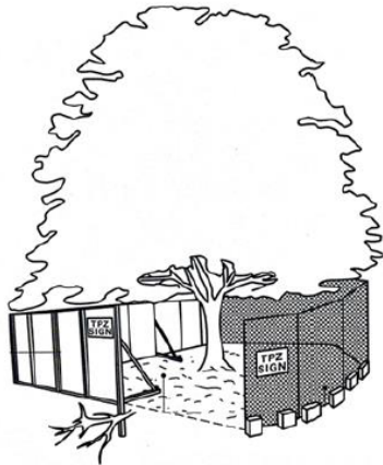
Tree protection fencing
