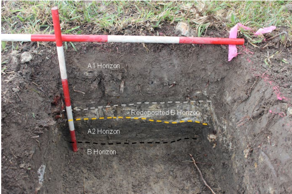
Figure 3.9 TU04, a characteristic Type 3 soil profile—scale bar segment is 100mm. (Source: GML 2021)
