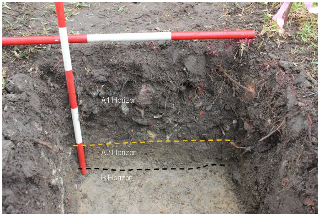
Figure 3.10 TU02, a characteristic Type 3 soil profile—scale bar segment is 100mm. (Source: GML 2021)
