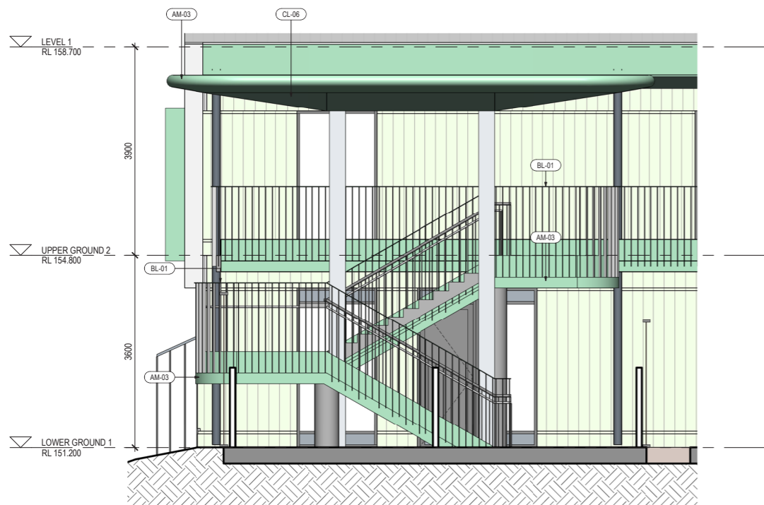
3 Typical Stair Elevation Scale: 1 : 50
