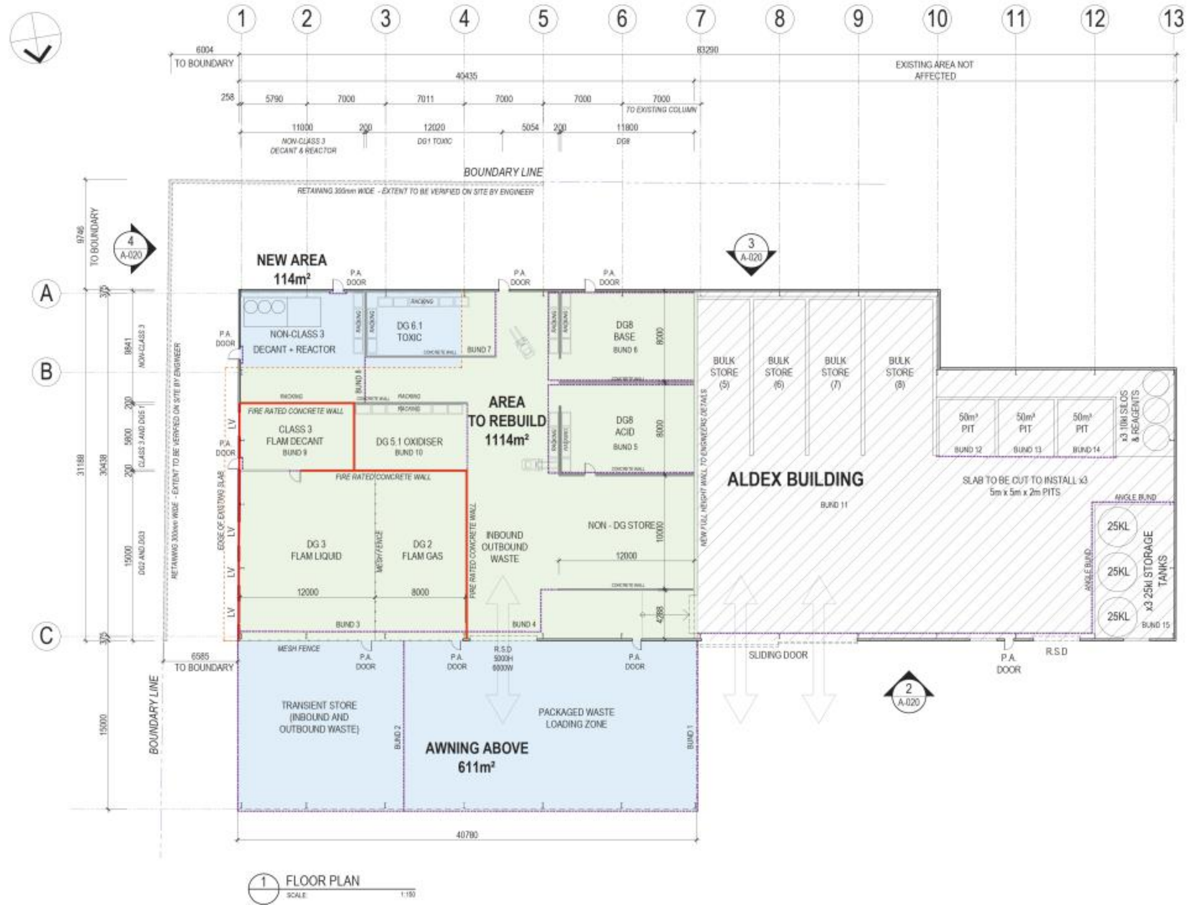
Figure 3-3: Proposed Waste Chemical Storage Area (Eastern End)
