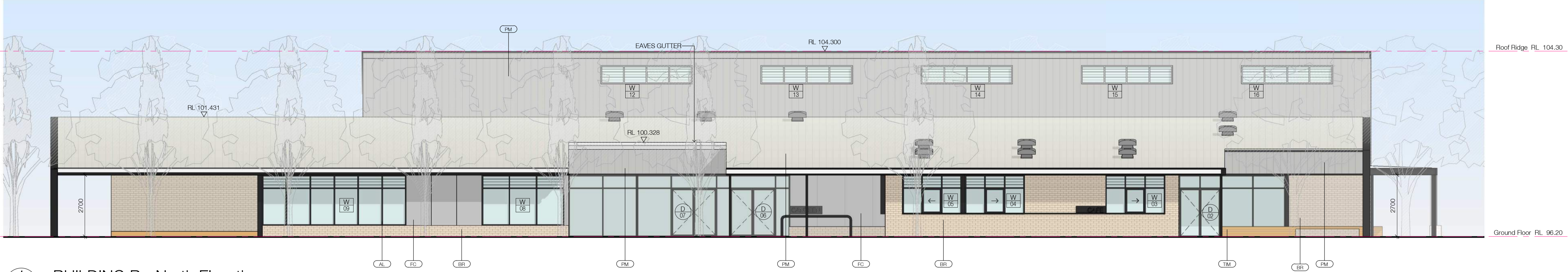
1 BUILDING B - North Elevation Scale 1 : 100
