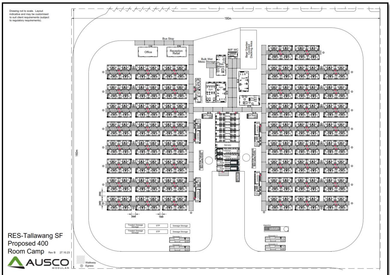
Figure 4.1: Proposed 400 Room Temporary Workers Accommodation
