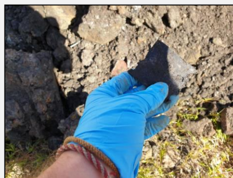
Photo 10: Asbestos-containing fibre cement sheeting sampled at TPI9 (AS001).
