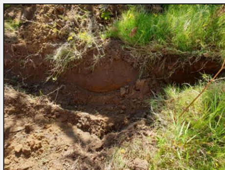
Photo 5: Overlying fill material observed at TP3.
