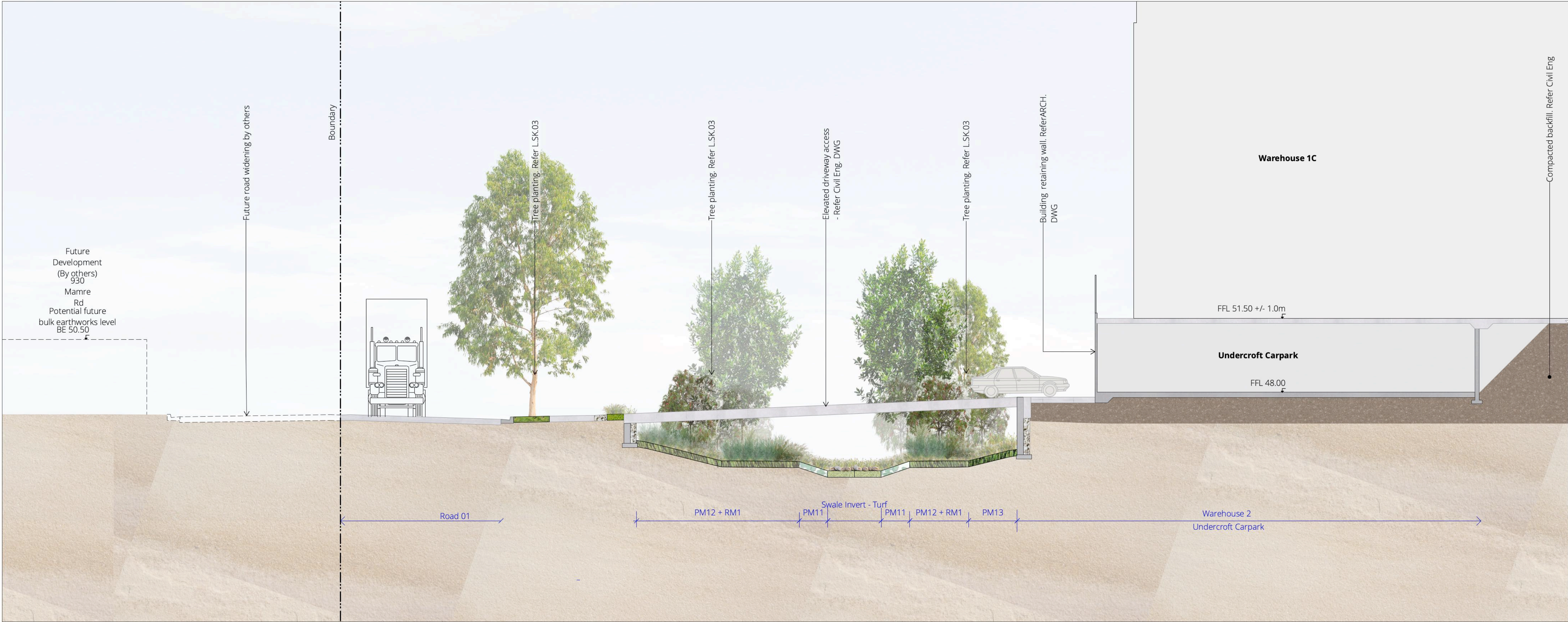
04 SECTION - SOUTHERN / BIORETENTION SWALE SCALE: 1:200@A1
