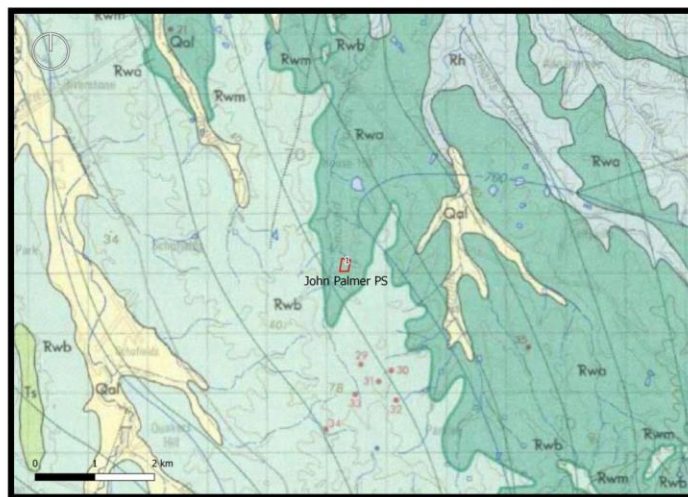
Figure 8: Geology Map for the John Palmer Public School. Rwa represents Dark-grey to black claystone-siltstone and fine sandstone-siltstone laminate (Clark and Jones 1991).
