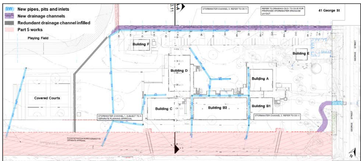
Figure 13 | Proposed on site flood mitigation works and stormwater infrastructure (Base source: Applicant's RtS)
