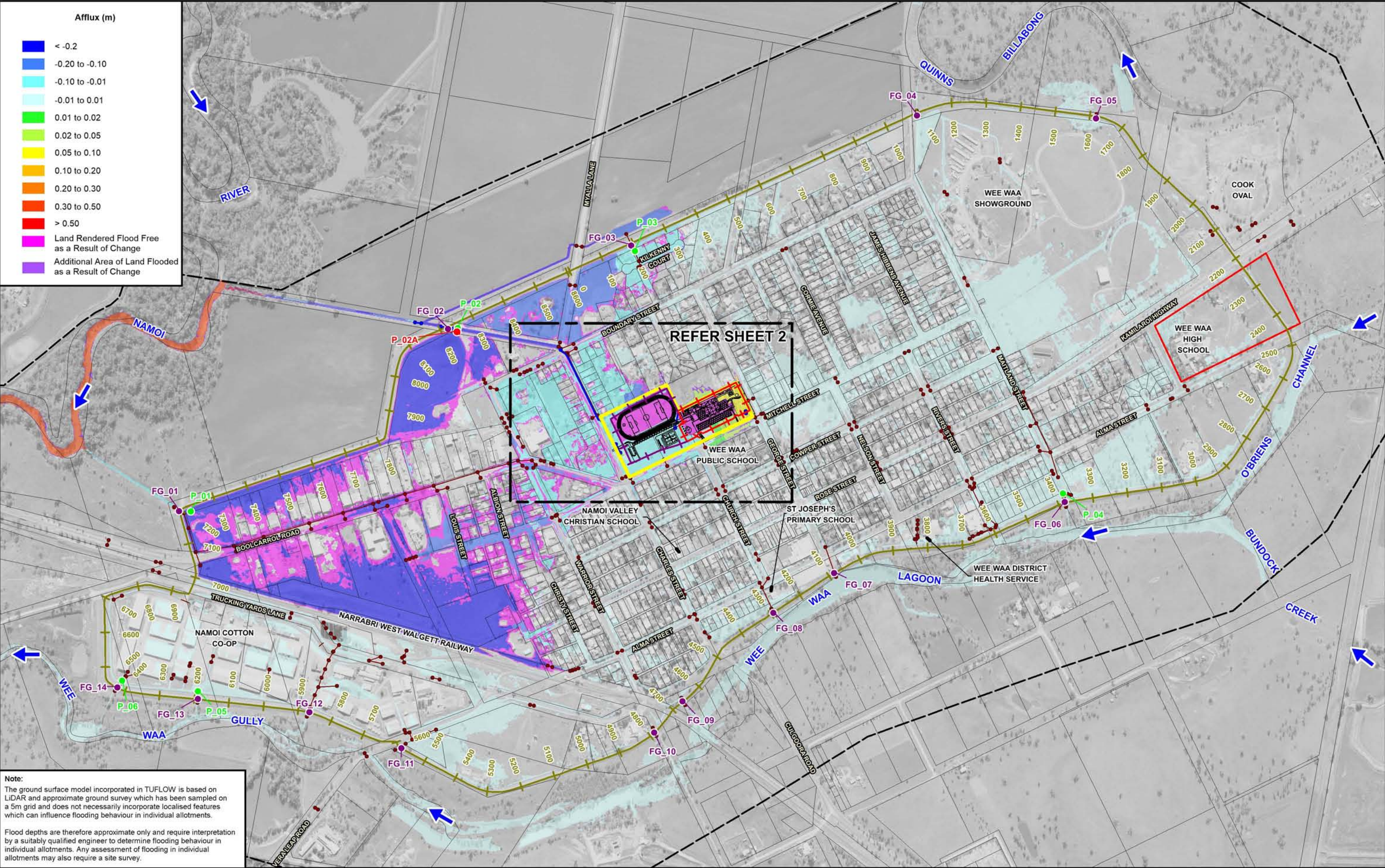
Figure 6.21 (Sheet 1 of 2) IMPACT OF PROPOSAL AND FMW ON FLOOD BEHAVIOUR INTERNAL TO TOWN LEVEE POST-10% INCREASE IN 1% AEP RAINFALL INTENSITY CONDITIONS
