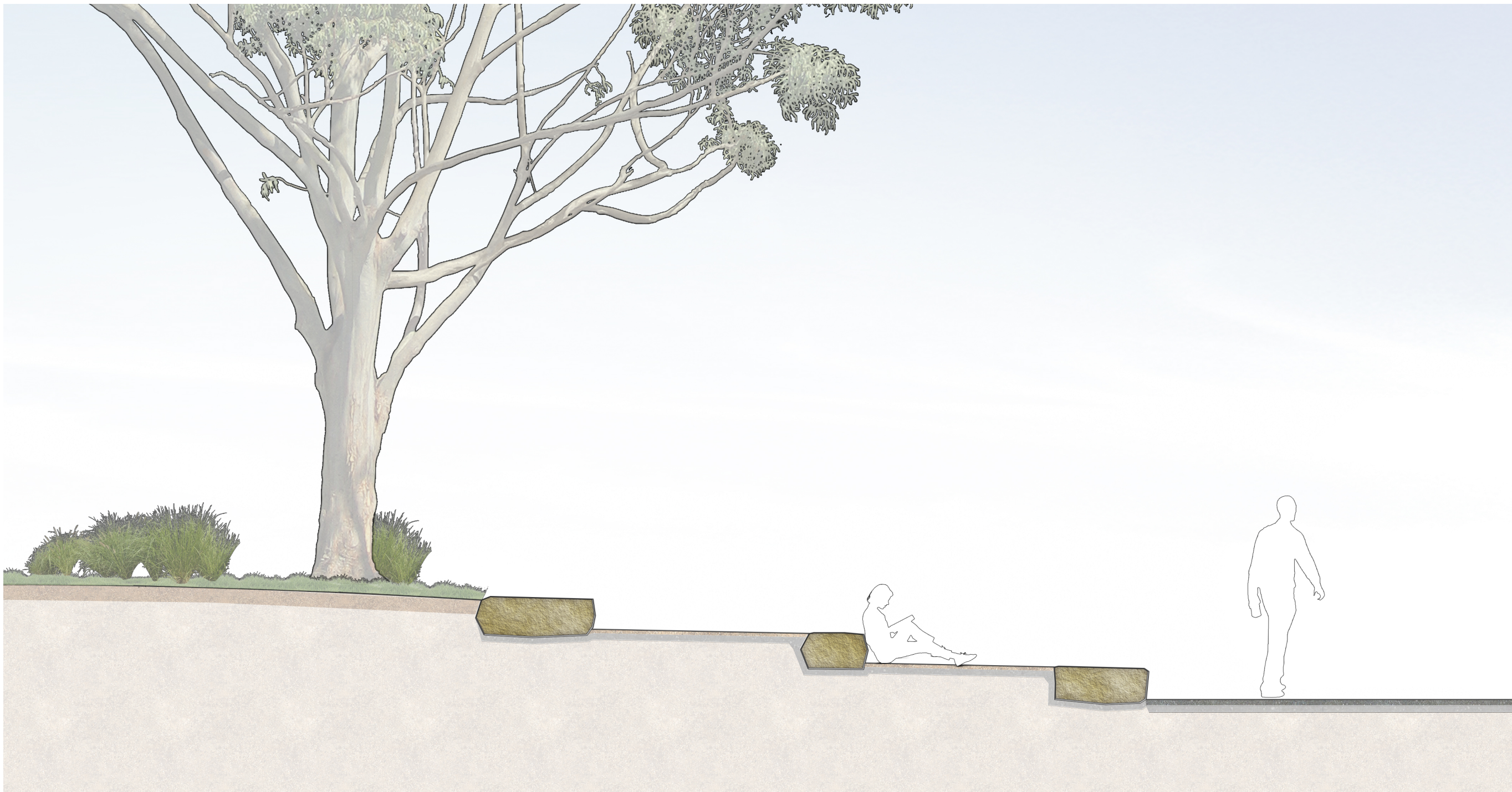
01 LP06 TYPICAL SECTION THROUGH INFORMAL RAISED SEATING IN COURTYARD Scale: 1:50
