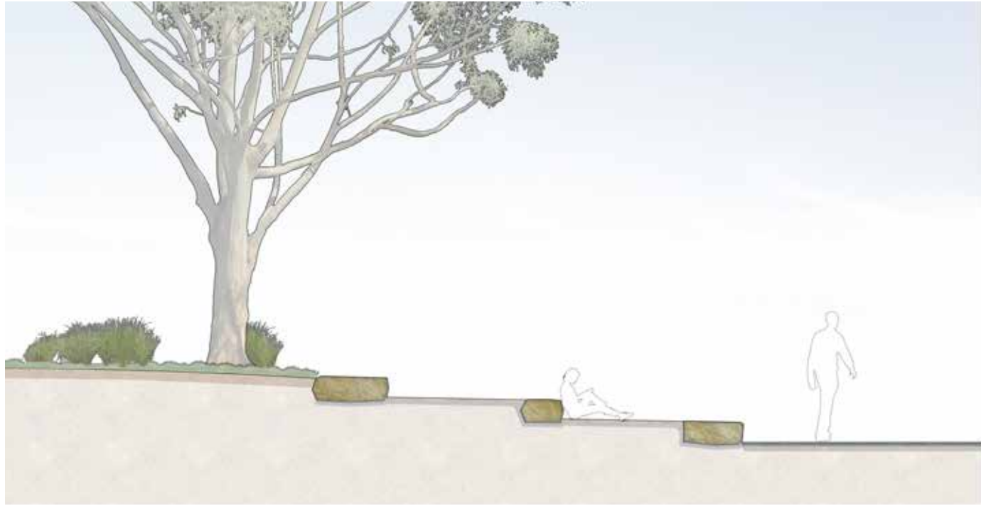
Indicative Cross Section A - A showing raised 'bleacher' stone edge in central courtyard - Scale 1:40@a3
