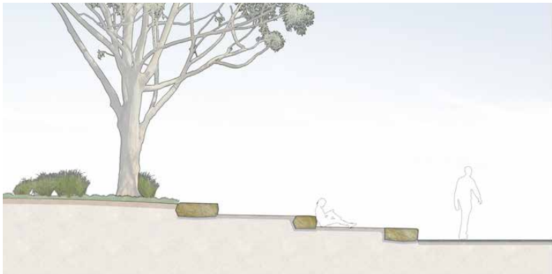
Indicative Cross Section A - A showing raised 'bleacher' stone edge in central courtyard - Scale 1:40@a3
