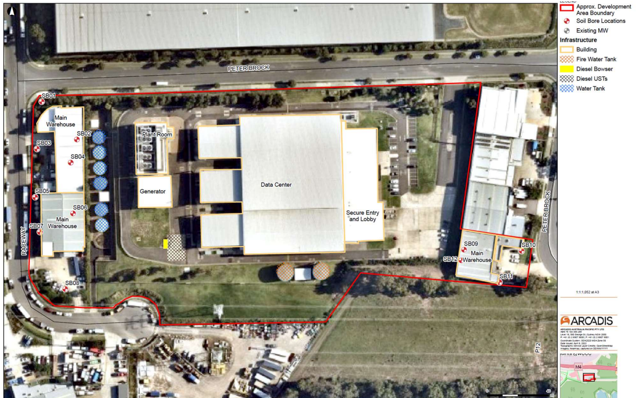
Figure 6.10: Site Contamination Sampling Locations (Source: Arcadis)
