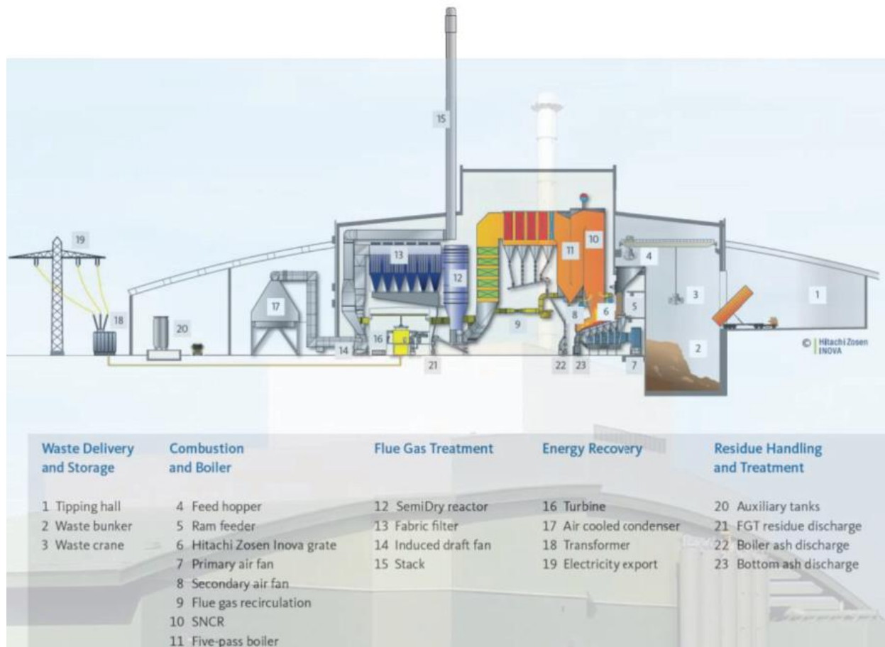
Figure 2: Schematic and main systems of the plant
