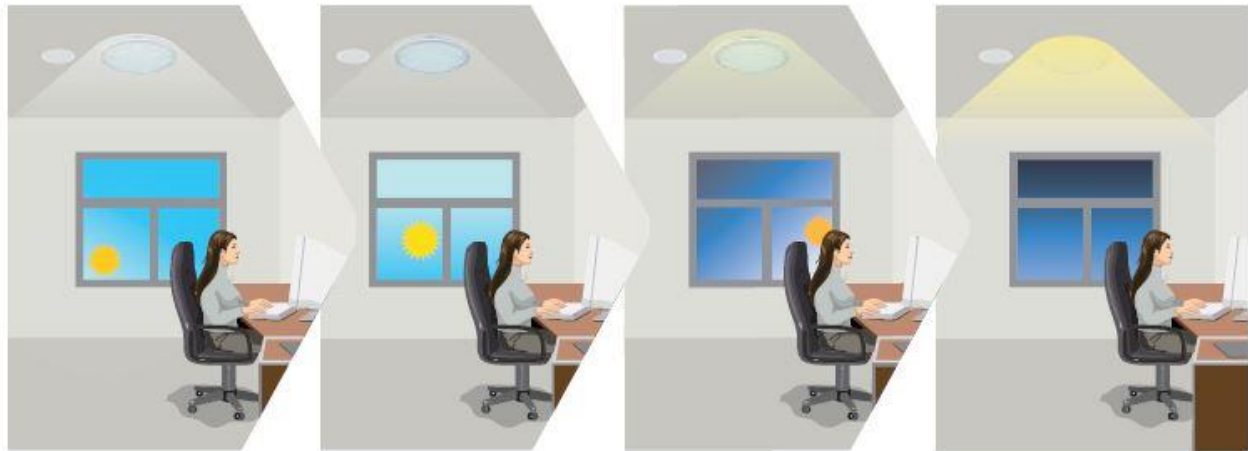
Figure 17: Daylight Harvesting over normal workday Source: ADM
