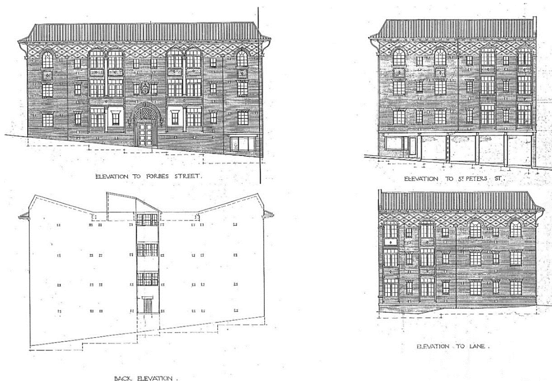
Figure 16 – Elevations of Wilkinson House, constructed in 1926. Note the terraced excavation which was required for the partial basement.
