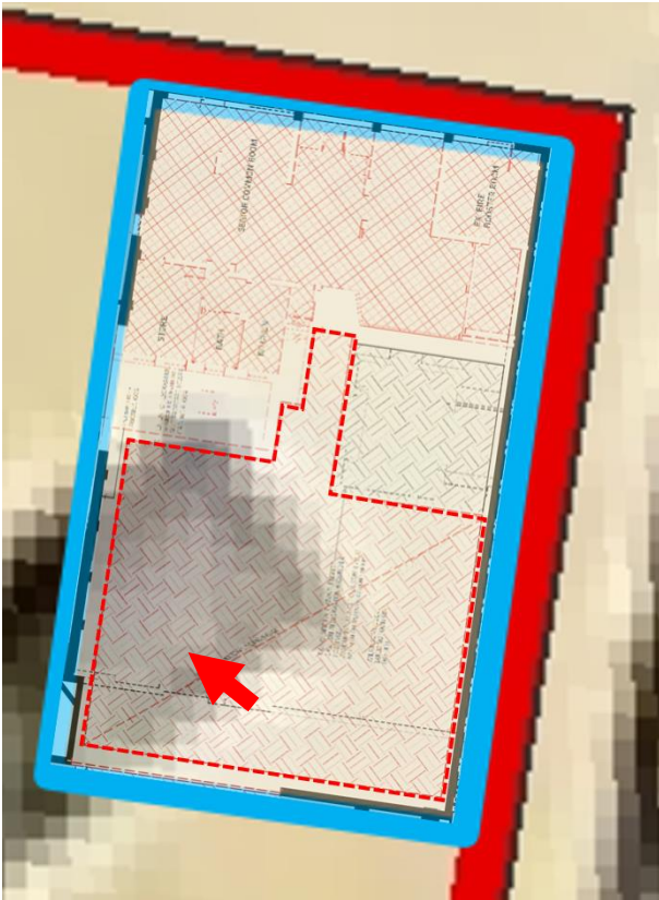
Figure 30 – Overlay of demolition plan on 1854 Woolcott and Clarke map indicating location of stone cottage (with arrow) relative to proposed excavation footprint (indicated with red dotted line).
