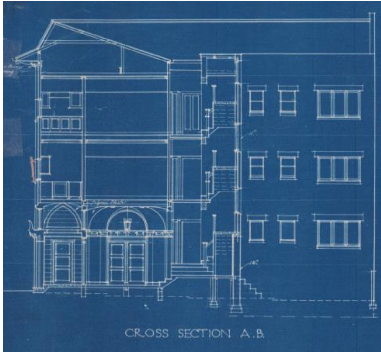
Figure 93 – Cross-section of the original design of the Gwydir Flats, 1926.
