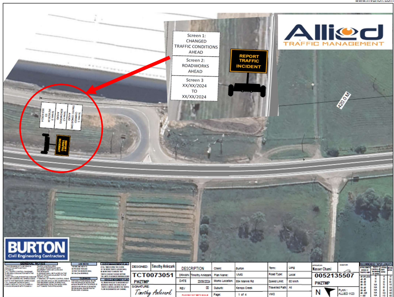
Figure 18 VMS for 884 to 924 Mamre Road – Sheet 1 of 3
