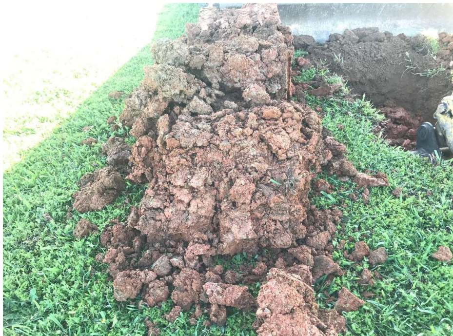
Photo 10 - Typical CLAY unit encountered
