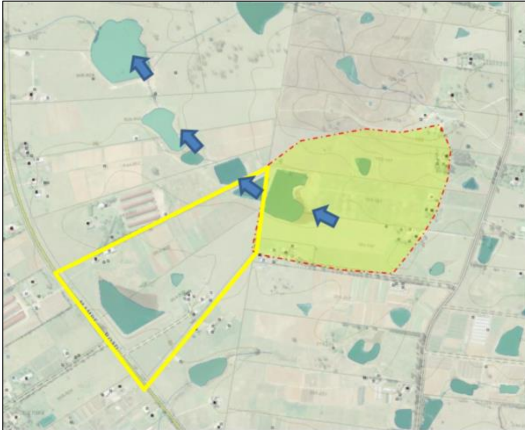
Figure 54 Upstream Contributing Catchment (Costin Roe 2021)
