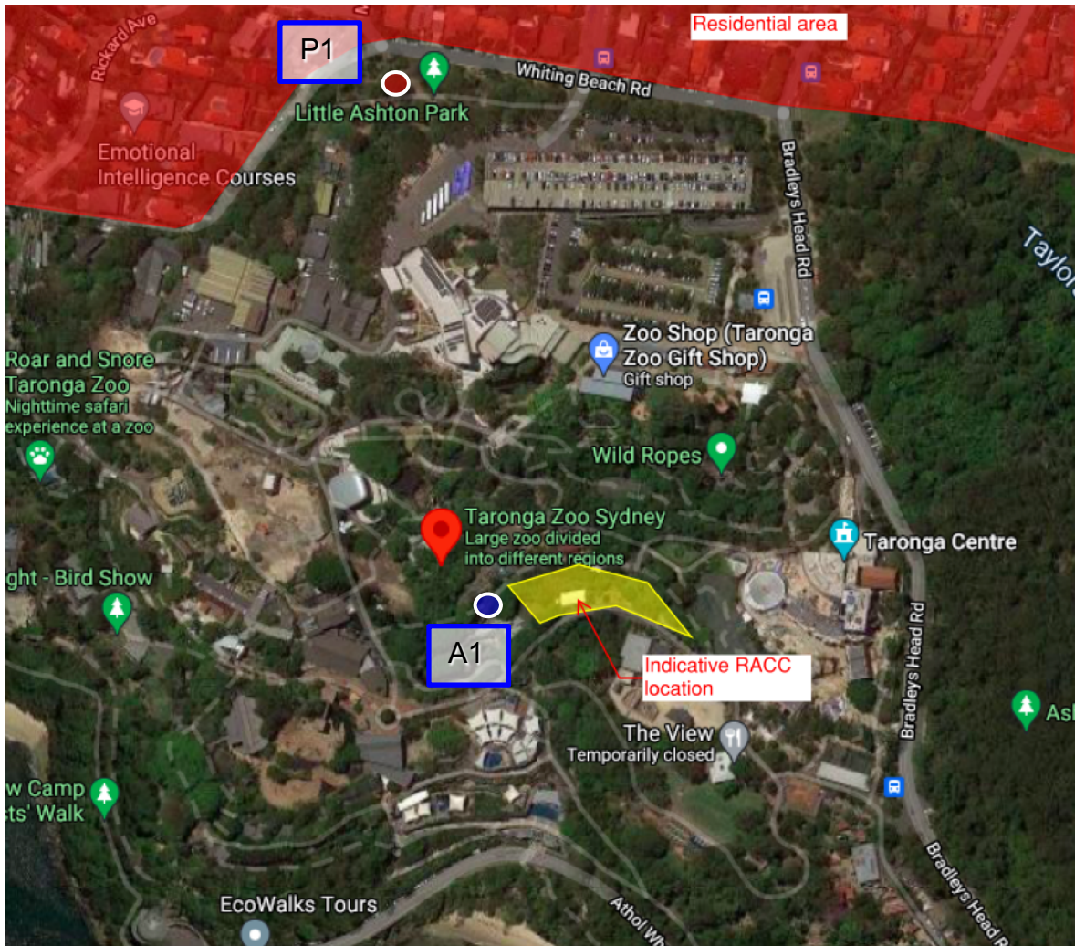
Figure 2: Location of proposed Reptile and Amphibian Conservation Centre (RACC) in relation to noise-sensitive receivers outside the zoo (residential receivers to the north).
