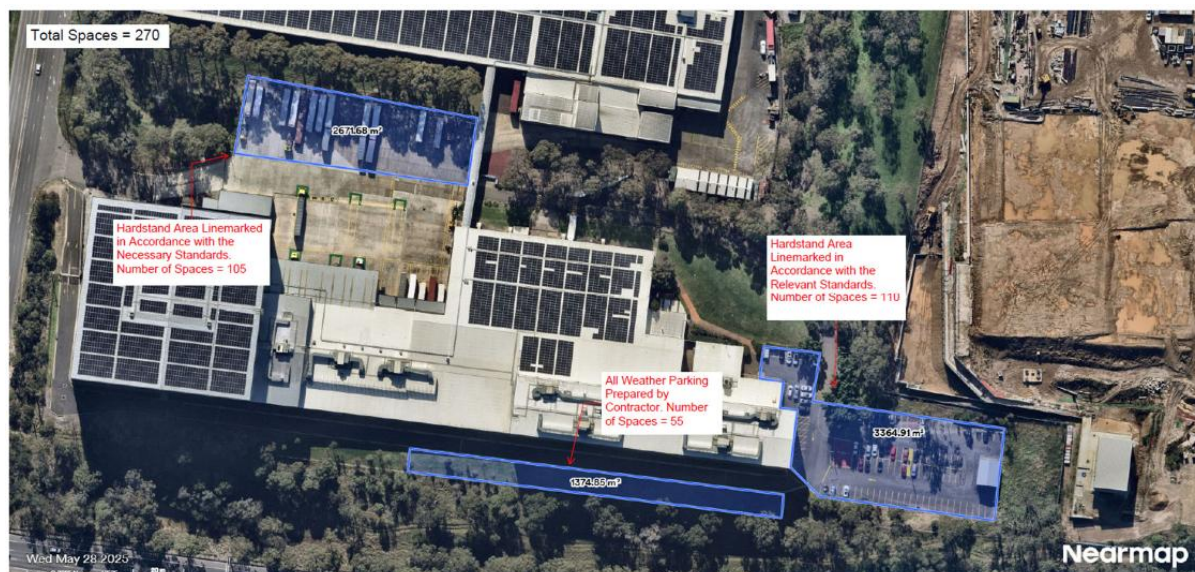
Figure 3 Temporary Carpark Space during Stage 2 Construction – sourced from TIA
