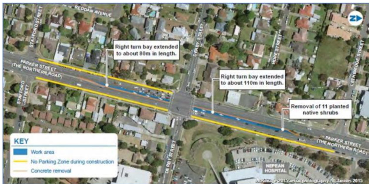
Figure 22 - Pinch Point upgrade at the Parker and Derby Street intersection
