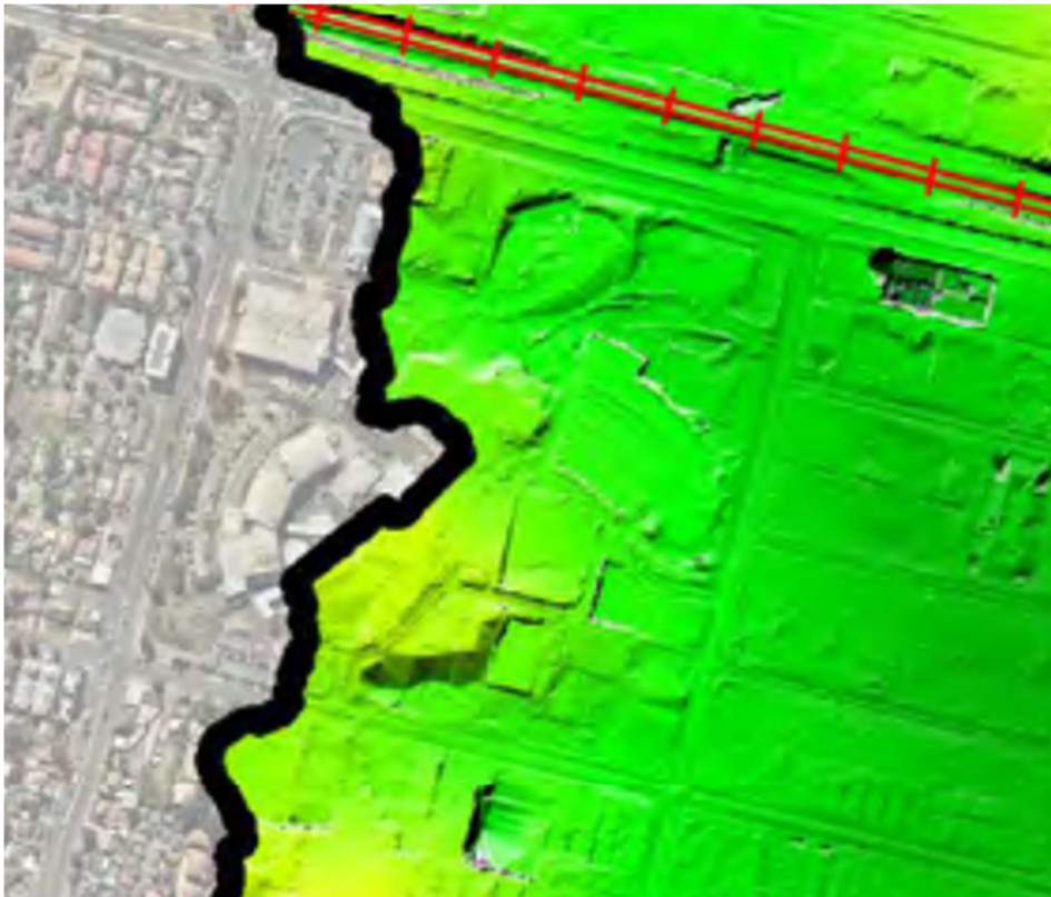
Figure 5-A – Surface Model Used in Flood Modelling (Catchment Simulation Solutions Floodplain Risk Management Study Draft 7-5-2021)
