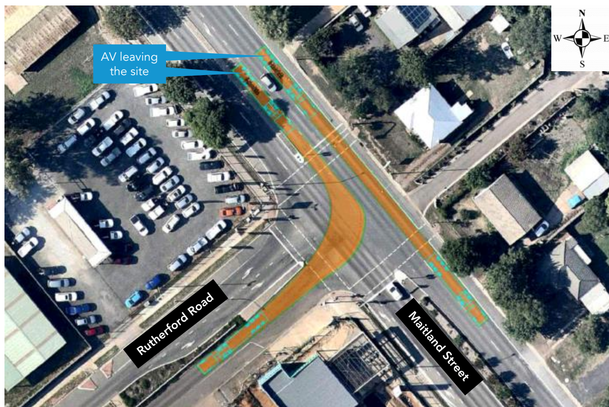
Figure 25 – AV leaving the site towards east via Maitland Street and towards north, south and west via Rutherford Road
