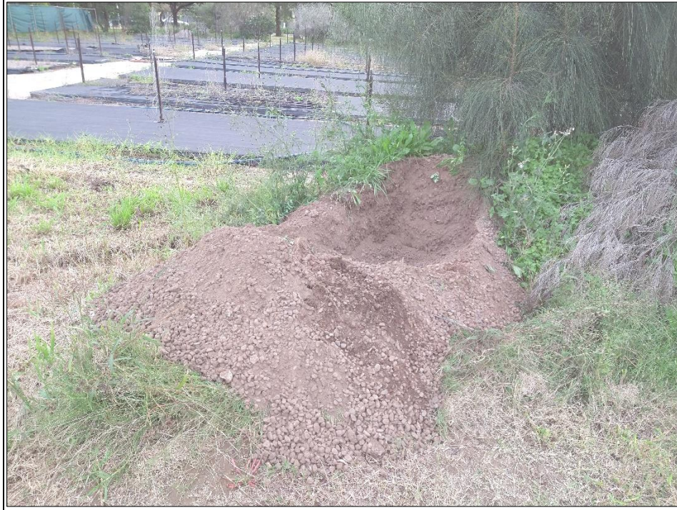
Figure 11: Stockpile 304 located in the central northern portion of the site, generally comprising silty sand and gravel.
