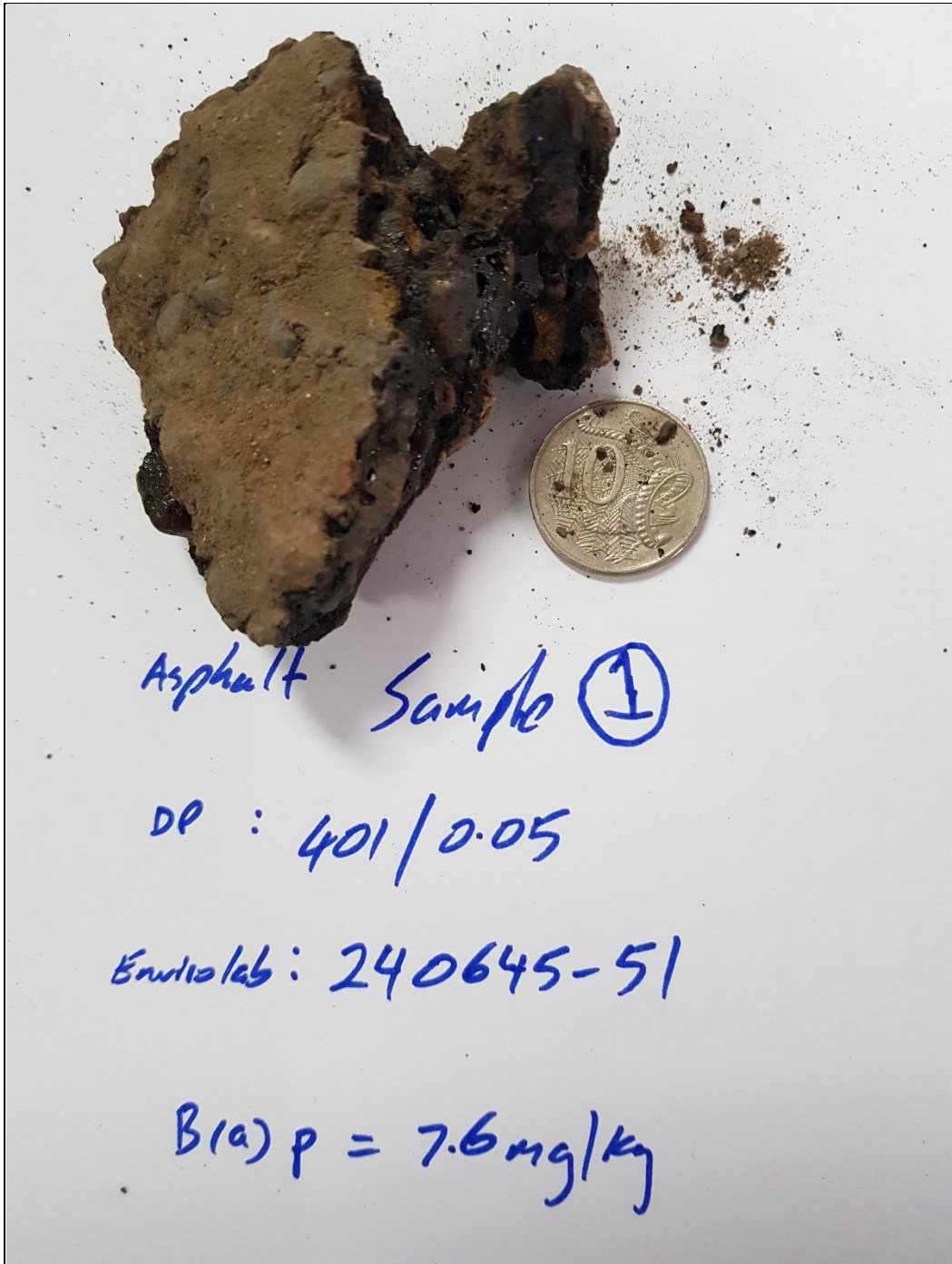
Figure 35: Photo of surface asphalt from test pit 401.
