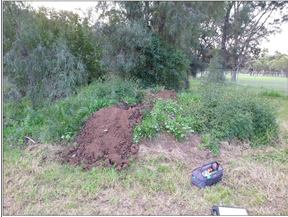
Figure 13: Stockpile 306 located in the central northern portion of the site, generally comprising silty sand and gravel and intermixed clay with trace asphalt.
