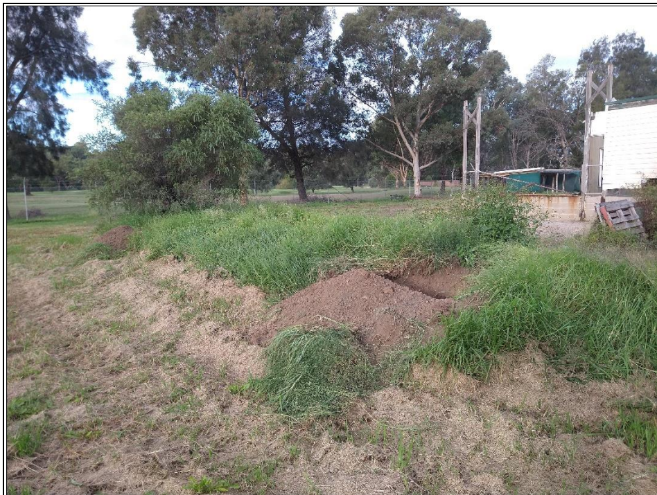
Figure 10: Stockpile 303 located in the central northern portion of the site, generally comprising silty sand and gravel.
