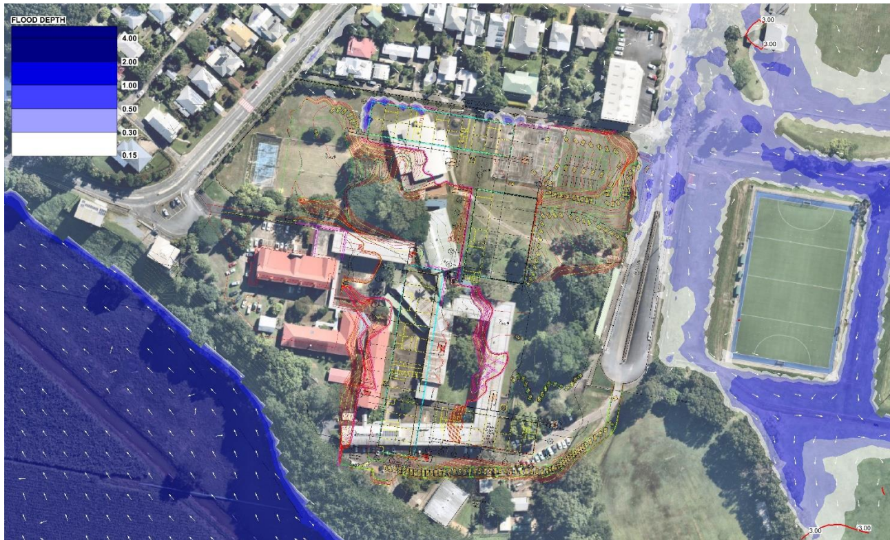
Figure 10 – 5% AEP Post Development Flood Levels and Depths
