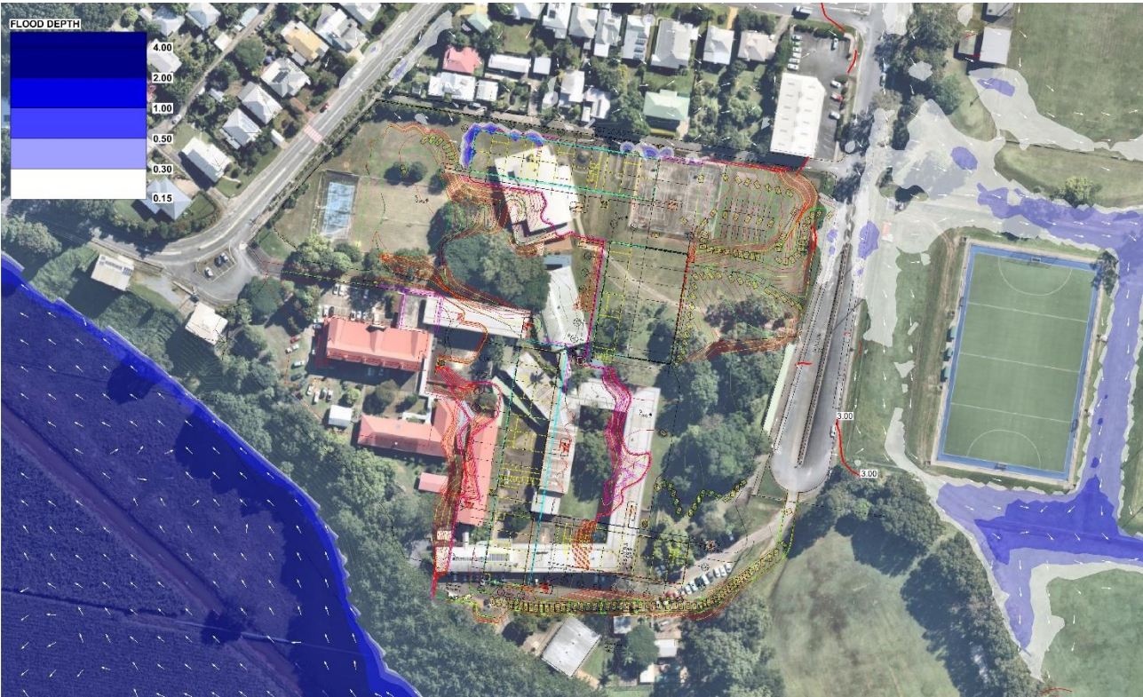
Figure 8 – 20% AEP Post Development Flood Levels and Depths
