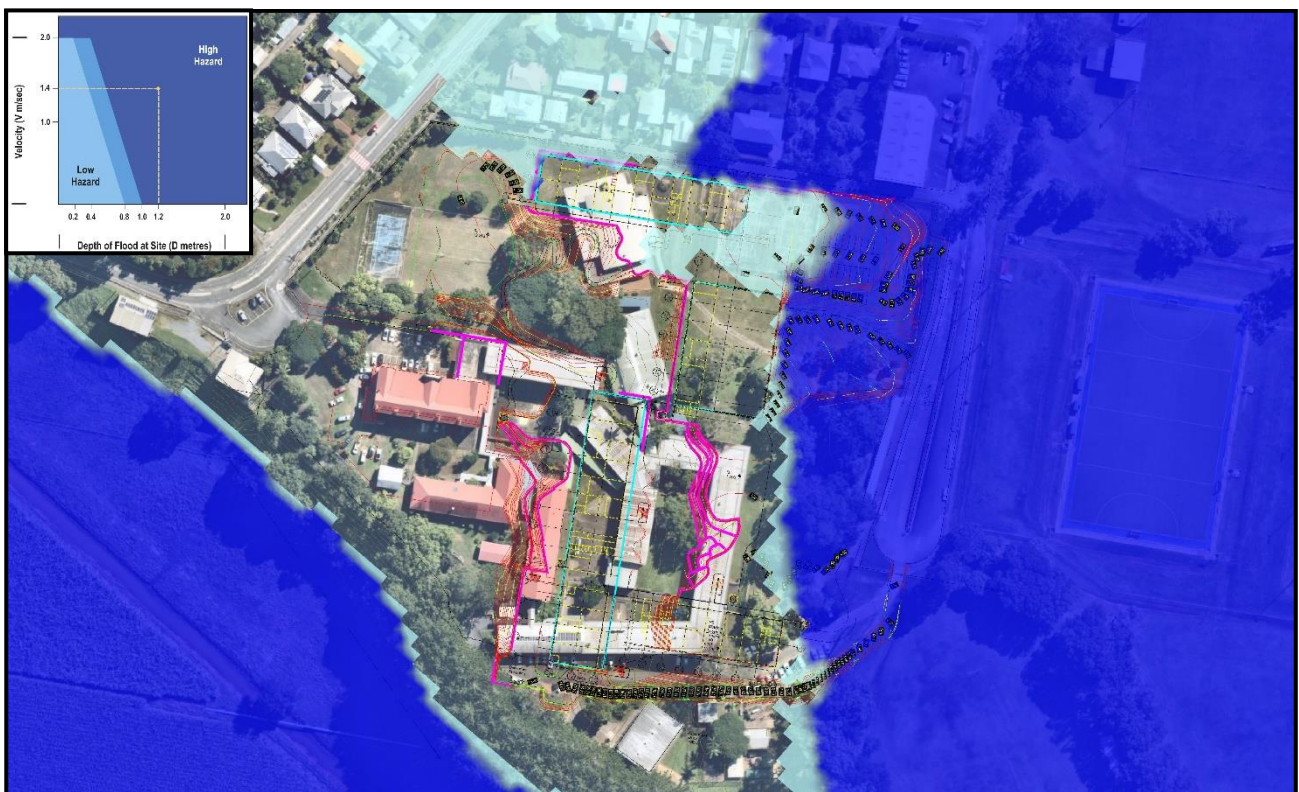
Figure 15 – 0.2% AEP Post Development Flood Hazard
