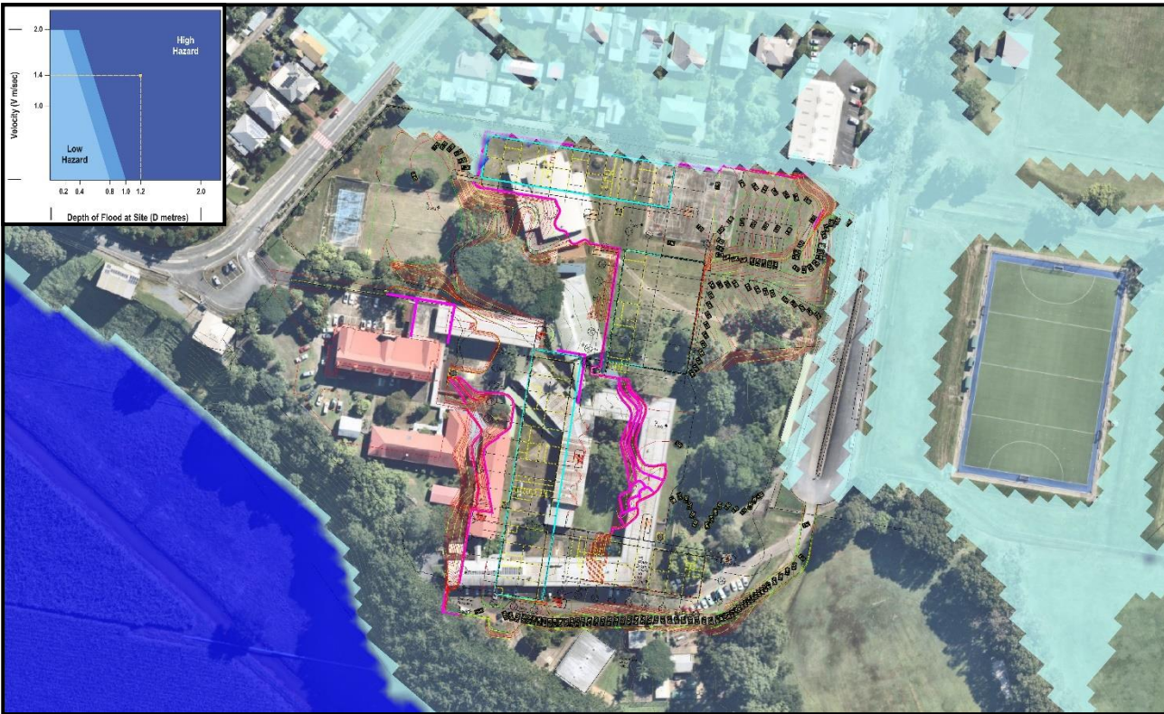
Figure 9 – 20% AEP Post Development Flood Hazard
