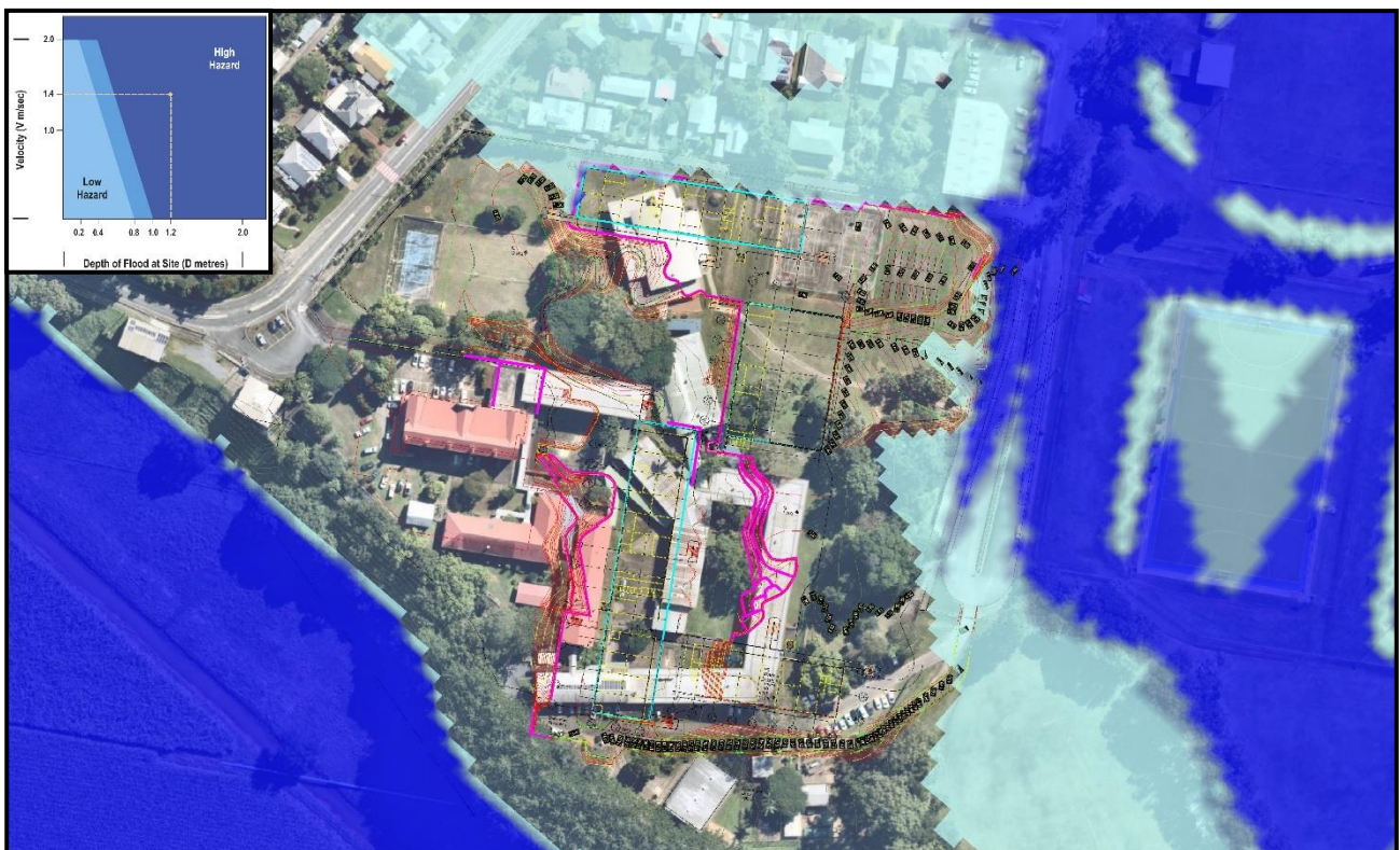
Figure 13 – 1% AEP Post Development Flood Hazard
