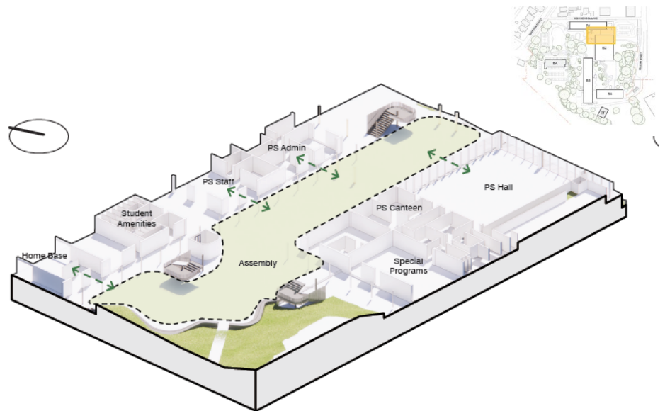
Figure 35 Circulation into/out of the primary school assembly area.
