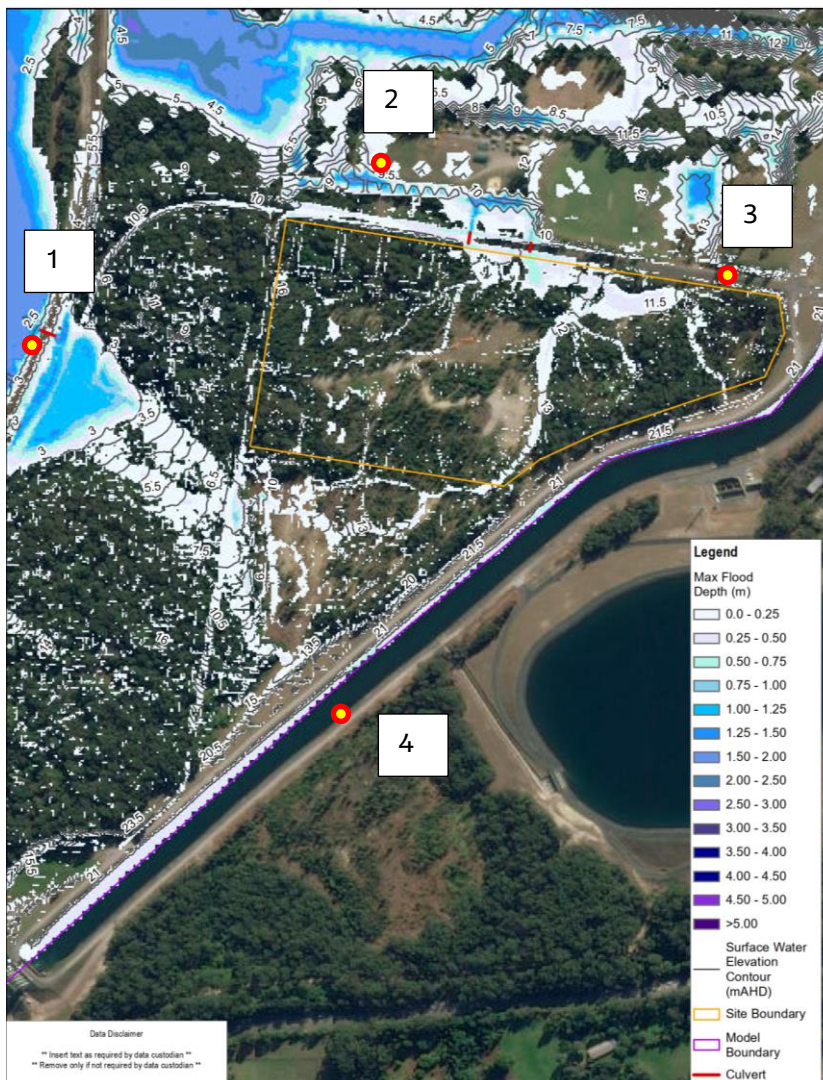
Figure 6-9: Flood level reporting locations (extracted from Figure 3-4 in GHD (2021 a)). (1% AEP flood shown)
