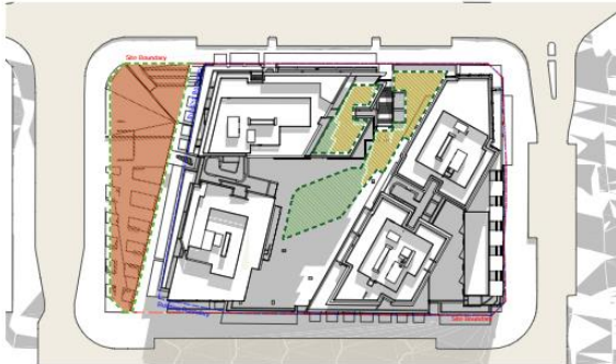
Figure 46: Communal area shadow diagram - 12:25pm (Source: Turner)
