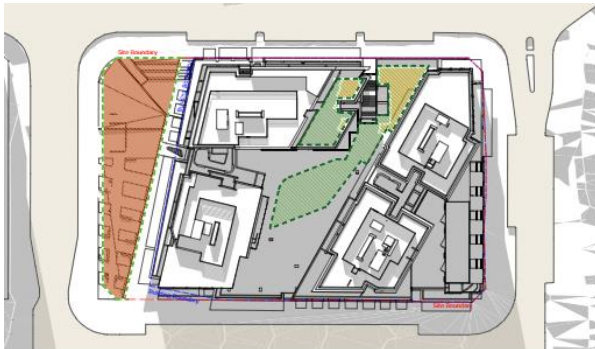
Figure 48: Communal area shadow diagram - 2pm (Source: Turner)
