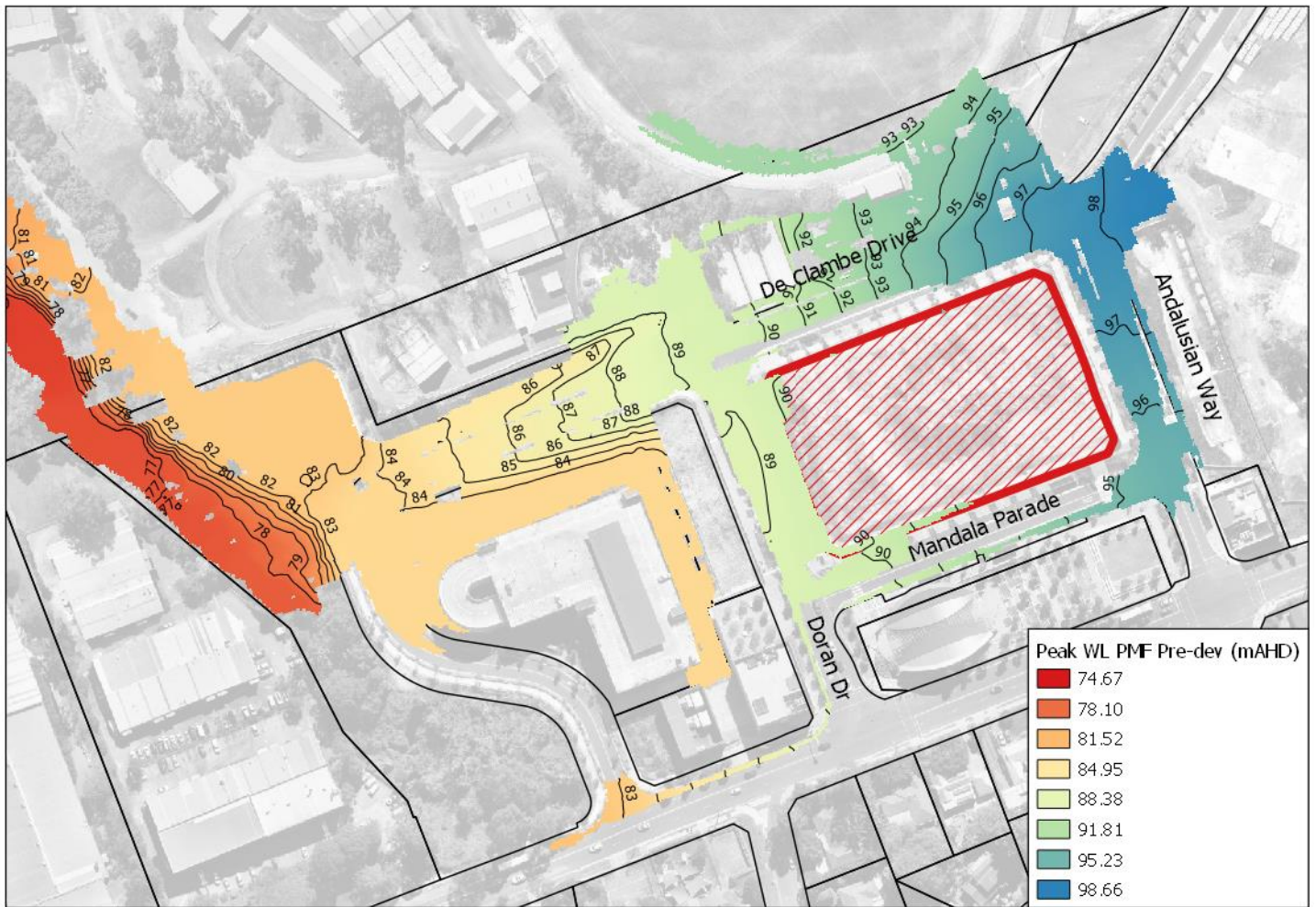
Figure 4.10 – Existing Scenario PMF Flood Level
