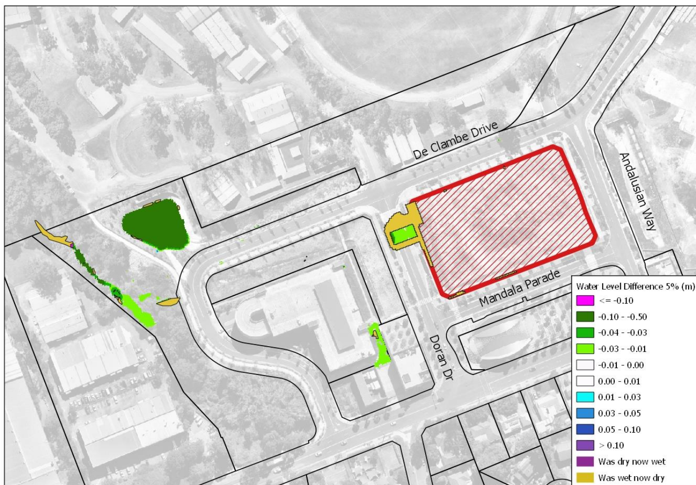
Figure 4.27 – Flood Level Difference – 5% AEP
