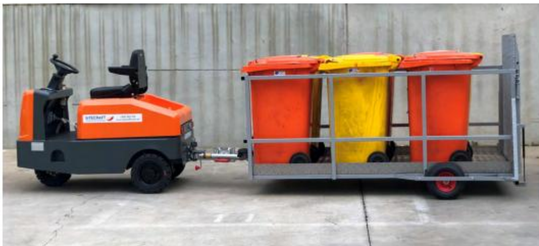
Optional steel / aluminium trailers for moving waste bins, linen trolleys, food trolleys, delivery boxes, etc ...
