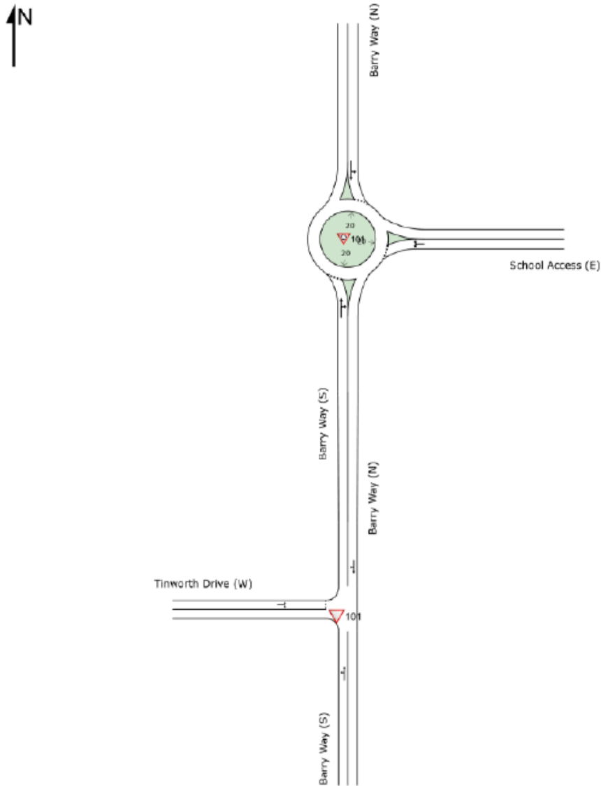
Figure 7-15 SIDRA Network Layout Source: Aurecon
