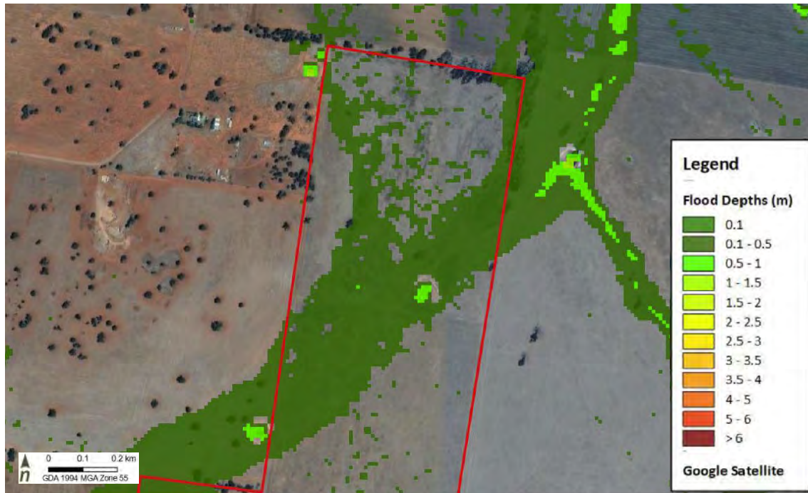
Figure 6.13 1% AEP flood depths close up of the northern area of the site (from Alluvium)
