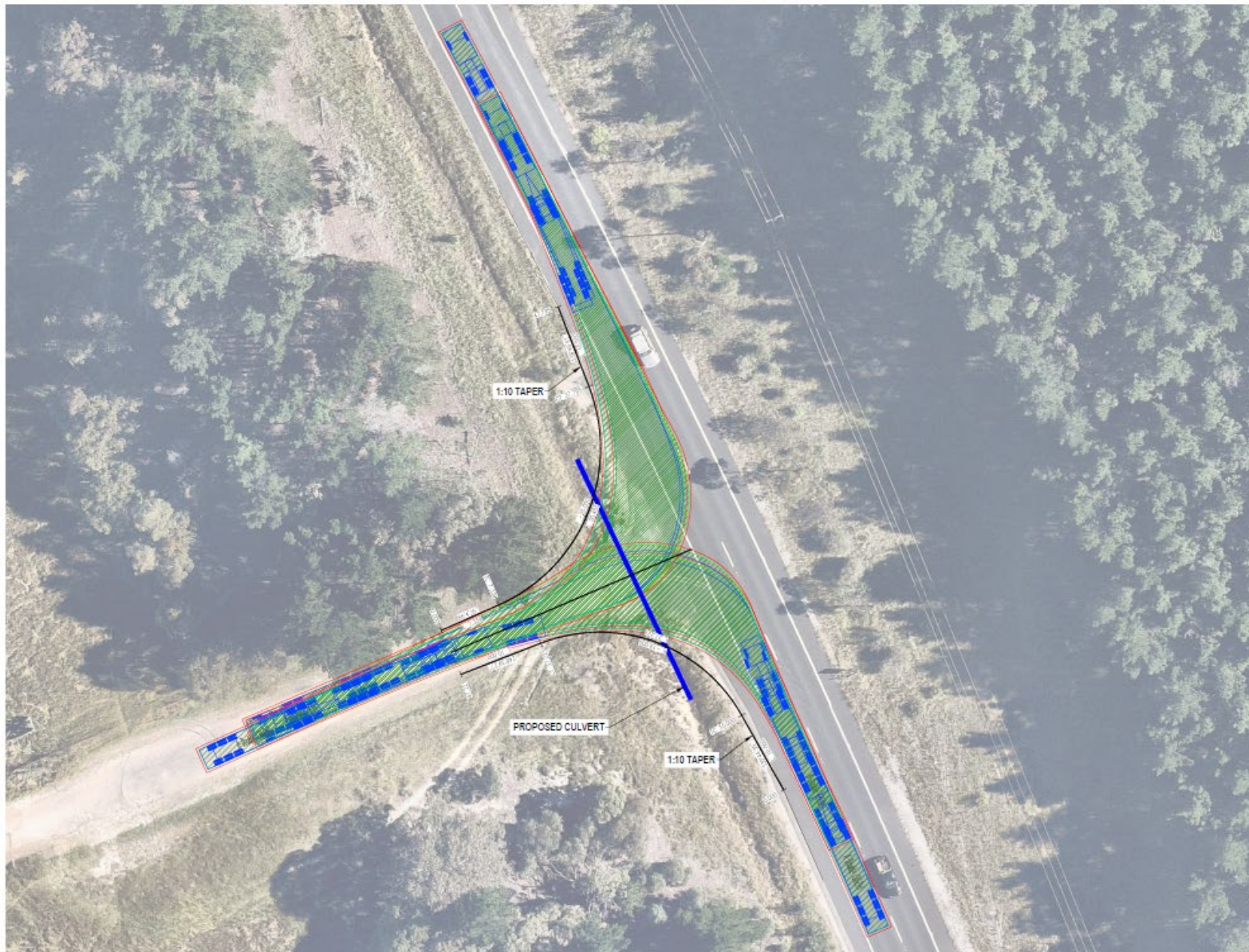
Figure 4-4 OSOM 36 metre Vehicle Swept Path
