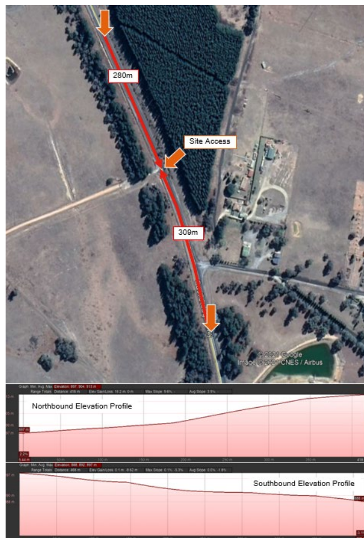
Figure 4-6 Access sight distances and longitudinal grades
