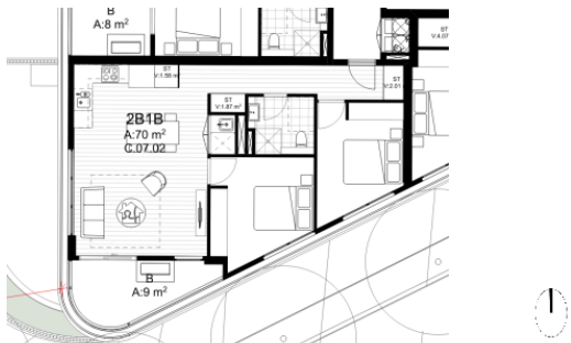
Fig.4E1.C1 9m2 balcony to 2-bedroom x 1-bathroom apartment (C.01.02 - C.08.02)
