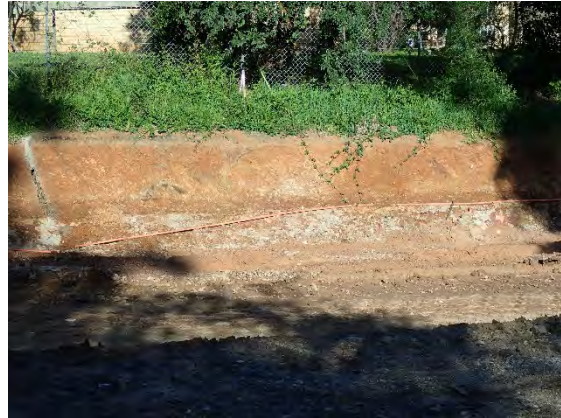
Figure 30 – Detail shot of section showing approximately 1m of red basal clay above a light grey plastic clay. Extremely shallow disturbed topsoil visible within rail corridor.
